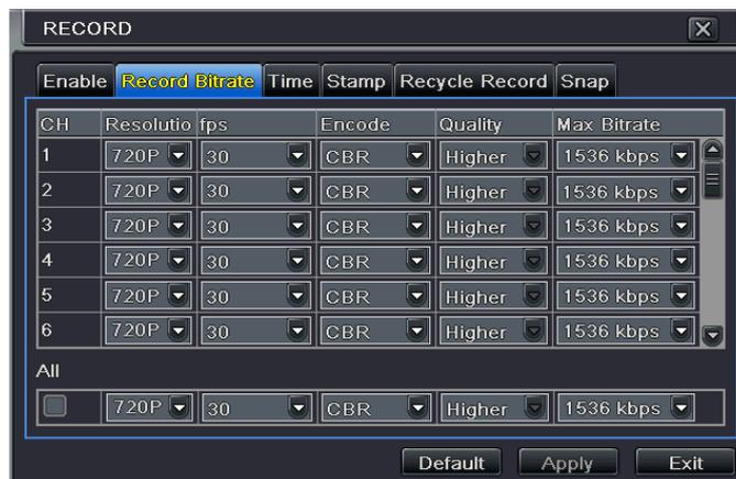
**Setup the DVR:** Set the FPS, resolution, quality, encode and max bitrate according to your recording requirements then click “Apply”.
