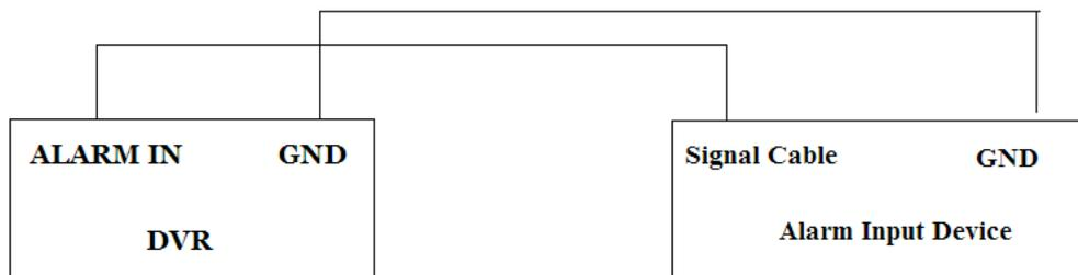
The alarm input is an open/closed relay. If the input is not an open/closed relay, please refer to the following connection diagram:
