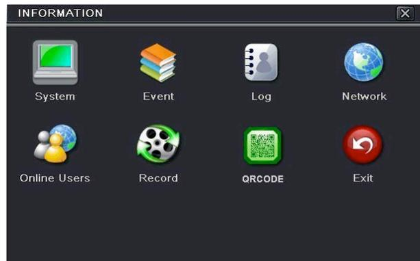
**System:** Check the hardware version, MCU version, kernel version, device ID, etc.
