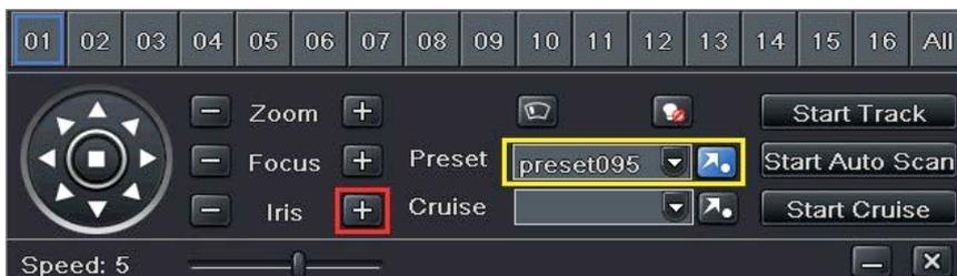
Double click “Iris +” to enable the menu of the PTZ camera. Use the directional wheel to move around the menu, then use “Iris+” as an enter command. Please refer to the user manual of the PTZ for more details.
