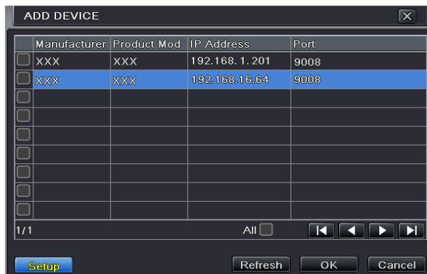
If the IP Camera is not in the same local network, you can select the device and click “setup” to modify the IP address of the searched device.
