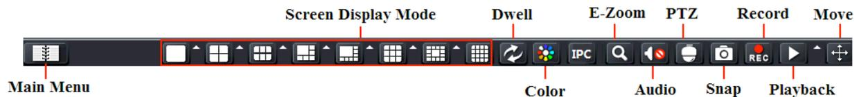
Click the right mouse or press ESC on the front panel and the control bar will be display at the bottom of the screen.
