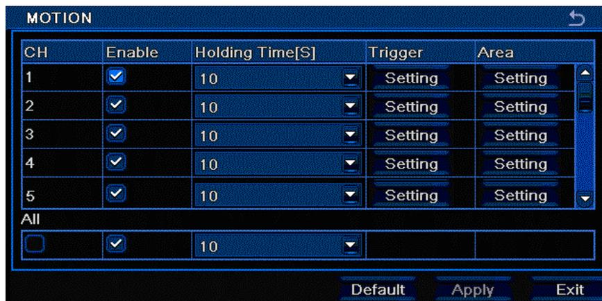
**Enable:** Left click the check box to enable motion triggered recording on a particular camera Channel. Remember you also have to schedule motion triggered recording as per section 3.4.2
