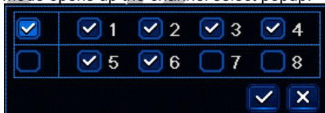
This allows you to select which cameras are displayed. Check the box relating to an individual camera, then click  button to confirm the setting.
