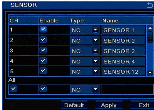
Left click tick box to enable an external alarm trigger on that particular camera channel. Under the “Type” column you can select whether the trigger is normally open, “NO”, or normally closed, “NC” in it’s resting state. There is the option to set all triggers to the same type by left clicking the “All” tick box and then clicking the “Type” drop down box to “NO” or NC”
