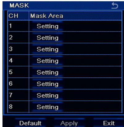
**To setup a mask area:** Left click "Setting". The screen will then show the live image from that camera. Starting at the top left of the area you wish to mask Left click and hold, then drag the mouse down and to the right. To remove an area double left click it. Once you are happy right click to return to the "Mask" sub menu and click "Apply"
