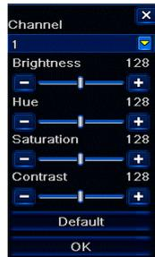
Individual parameters are changed by left clicking and dragging the slider for each element. Once you are happy click "OK". Default returns the DVR to a factory setting, not the setting as supplied by CCTV42 if it was supplied with a hard drive installed.
