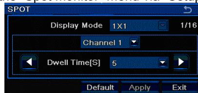
The spot monitor is only designed to display a single camera at a time. Select the camera from the drop down menu.
