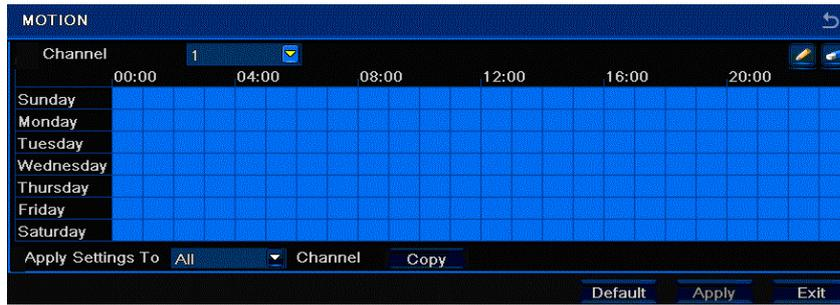
Setting up the schedule is identical to section 3.4.1 “Schedule”. Left clicking the default button in this section turns all the recording to ON.
