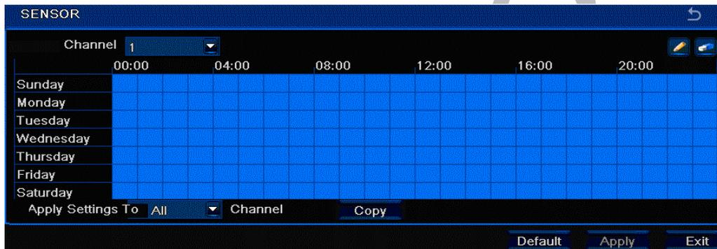
Setting up the schedule is identical to section 3.4.1 “Schedule”. Left clicking the default button in this section turns all the recording to ON.
