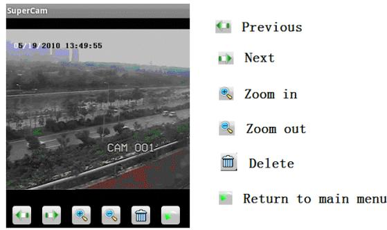
**Record playback:** Viewing previously recorded footage stored on the device
