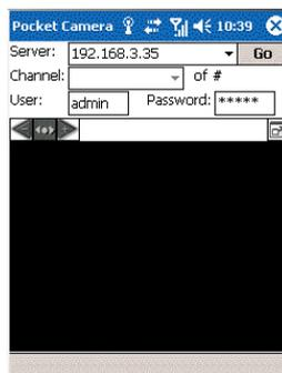
Input the web address of your CCTV system (probably your DDNS host name) in the “Server” box, the DVR unit’s User name in the “User” box (default admin) and the DVR unit’s password in the “password” box (default 123456). Click “Go” to log on to your CCTV system. You will be able to see a camera image from your system if you are successful.
