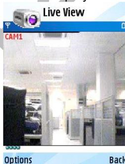
In Live View selecting "Options" allows you to change camera view, take Snap images, control PTZ cameras and so on.
