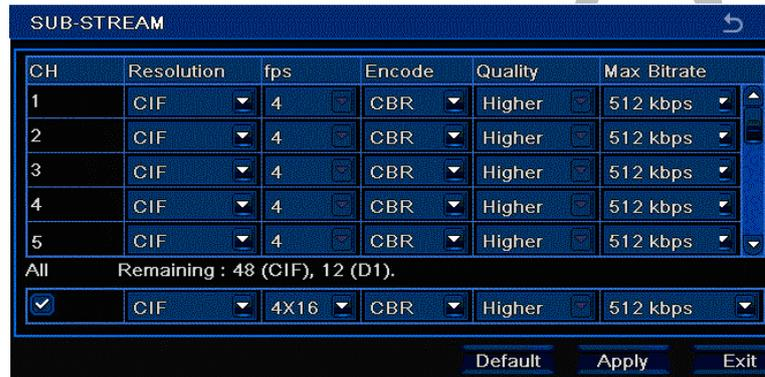
To make an alteration left click the chosen parameter and make your selection from the drop down menu the left click the "Apply" button. You can change all the camera channels by checking the "All" tick box using a left click of the mouse, make your selections from the menu drop down boxes then click the "Apply" button.
