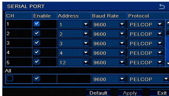
**Enable:** left click the check box to enable PTZ camera control on that particular camera channel.
