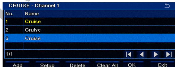
Left click the "Add" button to create a cruise or tour itinerary. Once highlighted left click the "Setup" button to open the cruise preset sub menu. You can create up to 8 pre-set cruises. To remove a cruise left click either the name or number, then left click the "Delete" button. Left Clicking the "Clear All" button removes all the cruises for that camera channel.
