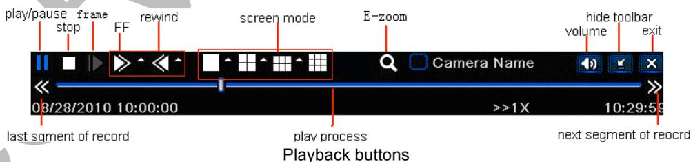
During playback it is possible fast forward, rewind, pause and single frame advance (this option becomes available when you pause the footage) by left clicking the respective button. You can also change the number of cameras being displayed by left the different screen mode buttons.
