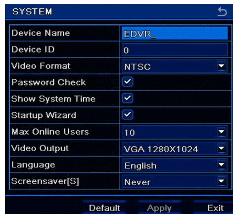
In this interface user can setup the DVR name, DVR ID number, video format (NTSC, PAL), maximum number of online users, Video Output (VGA, BNC), language, screensaver and so on.
