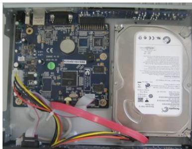
Step 3: Screw the HDD as below.
