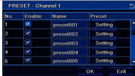
**Enable:** Left click the check box to enable specific preset points (1-128). There is no need to uncheck points which are unused.
