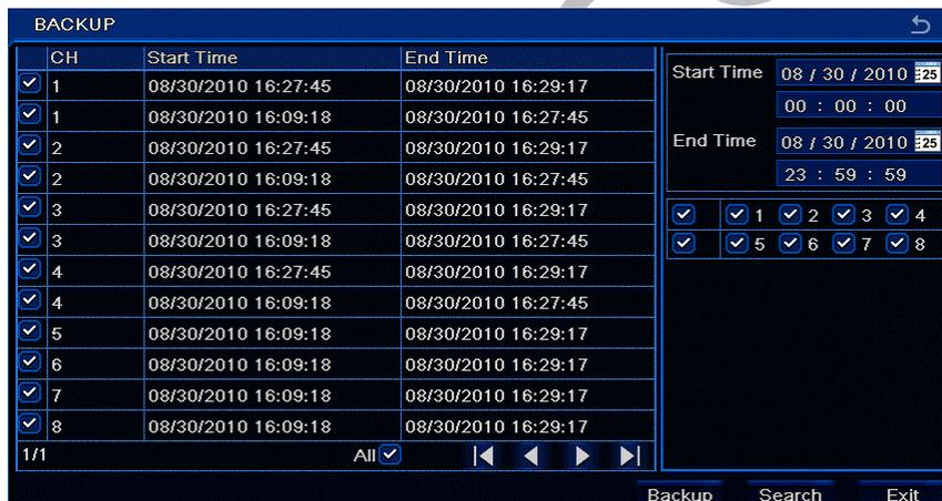
Once you are happy with the file block ensure you have inserted a storage device (memory stick) left click it's tick box remembering to uncheck the “All” tickbox first if it is checked, and then left click the “Backup” button.
