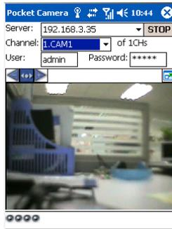
Camera 1 is the default channel after login. Change the camera using the scroll down “Channel” menu.
