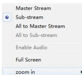
Sub-stream / master stream: The system2 DVR from cctv42 features dual streaming which allows you to compensate for lower bandwidth internet connection or make best use of higher bandwidth internet connection. By default the control panel displays the sub-stream (lower quality) feed. You can change the stream from this dropdown menu.
