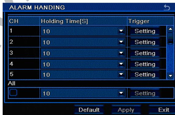
Left click to select the hold time in seconds, the time a trigger stays on for. Left click the "Trigger" button and a menu box will open.
