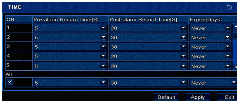
**Pre-alarm record time and Post-alarm record:** Left click the respective box then select from the drop down menu. Time is in seconds.
