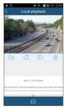
Slide the timeline to select the required playback time. A green block indicates manual record. Turning your phone can make the local playback display in landscape mode.
